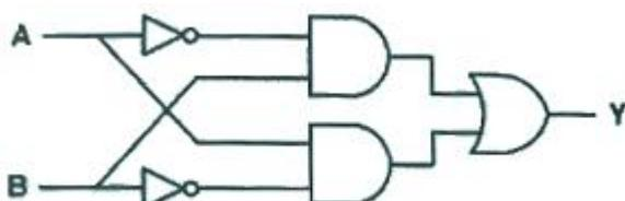
$$\textcircled{1} \quad Y = A\bar{B} + \bar{A}B \quad \textcircled{2} \quad Y = \bar{A}B + \bar{A}\bar{B}$$
