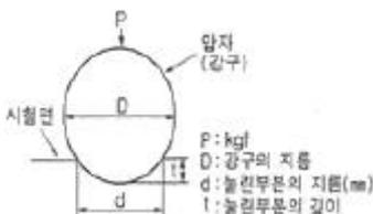
$$\text{1 } H_B = \frac{P}{\pi D l} \qquad \text{2 } H_B = \frac{P}{5\pi D l}$$
