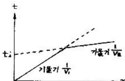
$$\text{① } Z = \frac{t_i}{2} \frac{V_1 V_2}{\sqrt{V_2^2 - V_1^2}}$$
