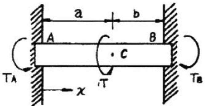
$$\begin{array}{ll} ① \frac{d\theta}{dx} = \frac{T}{GI_p} & ② \frac{d\theta}{dx} = \frac{T_A}{GI_p} \\ ③ \frac{d\theta}{dx} = \frac{T_B}{GI_p} & ④ \frac{d\theta}{dx} = \frac{T \cdot x}{GI_p} \end{array}$$
