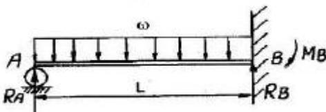
$$\textcircled{1} \quad R_A = \frac{4}{7} \omega L, \quad R_B = \frac{3}{7} \omega L$$
