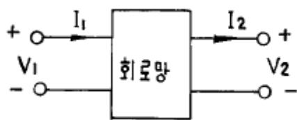
$$\textcircled{1} \quad A = \left| \frac{V_1}{V_2} \right|_{I_2=0}, \quad C = \left| \frac{I_1}{V_2} \right|_{I_2=0}$$
