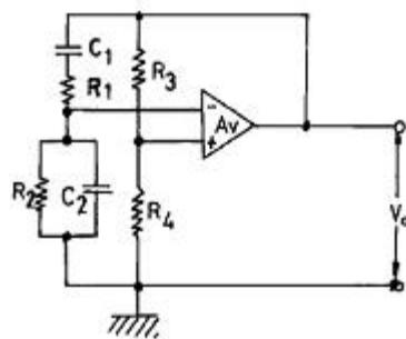
$$\textcircled{1} \quad f = \frac{1}{2\pi \sqrt{C_1 R_1 C_2 R_2}}$$
