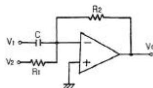
$$\textcircled{1} \quad -R_2 C \frac{dV_1}{dt} - \frac{R_2}{R_1} V_2$$
