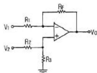
$$\textcircled{1} \quad -\frac{R_F}{R_1}V_1$$
