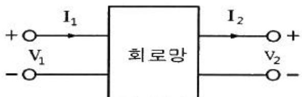
$$\textcircled{1} \quad A = \frac{V_1}{V_2}|_{I_2=0}, C = \frac{I_1}{V_2}|_{I_2=0}$$
