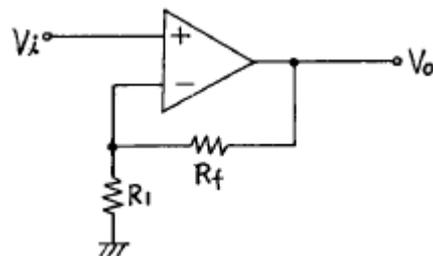
$$\begin{aligned} \textcircled{1} \quad V_o &= \frac{R_f}{R_1} V_i & \textcircled{2} \quad V_o &= -\frac{R_f}{R_1} V_i \\ \textcircled{3} \quad V_o &= -(1 + \frac{R_f}{R_1}) V_i & \textcircled{4} \quad V_o &= (1 + \frac{R_f}{R_1}) V_i \end{aligned}$$
