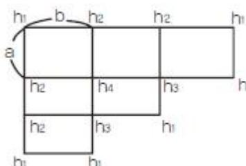
$$\text{① } V = \frac{ab}{4} (\Sigma h_1 + 3\Sigma h_2 + 2\Sigma h_3 + 4\Sigma h_4)$$
