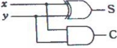
$$\begin{aligned} S &= x + y, \quad C = x \cdot y \\ \textcircled{1} \quad &S = x + y, \quad C = x - y \\ \textcircled{2} \quad &S = \bar{x} \cdot y + x, \quad C = x + y \\ \textcircled{3} \quad &S = x \cdot \bar{y} + \bar{x} \cdot y, \quad C = x \cdot y \end{aligned}$$
