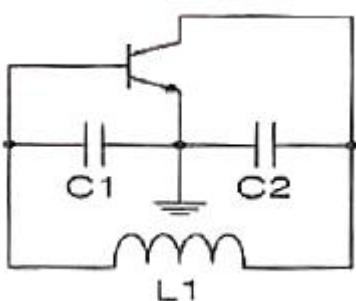
$$f_o = \frac{1}{2\pi \sqrt{L(\frac{C_1 + C_2}{C_1 C_2})}}$$
