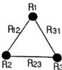
$$\textcircled{1} \quad R_1 = \frac{1}{2}(R_{12} + R_{31} - R_{23})$$
