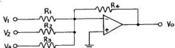
$$V_1 = 0.2 \text{ [V]}, V_2 = 0.3 \text{ [V]}, V_3 = 0.4 \text{ [V]}, R_1 = R_2 = R_3 = 1 \text{ [K}\Omega\text{]}, R_4 = 5 \text{ [K}\Omega\text{]}$$
