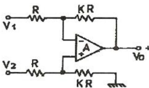
①  $V_o = K(V_2 - V_1)$       ②  $V_o = K V_2 - (K + 1) V_1$
