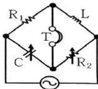
$$\textcircled{1} \quad \frac{C}{R_1} = R_2 L \quad \textcircled{2} \quad \frac{L}{R_1} = R_2 C$$
