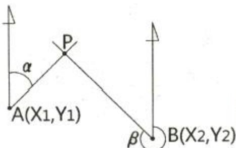
$$\begin{array}{l} \textcircled{1} \quad S = \frac{(Y_2 - Y_1)\sin\beta - (X_2 - X_1)\cos\beta}{\sin(\alpha - \beta)} \\ \textcircled{2} \quad S = \frac{(Y_2 - Y_1)\sin\beta + (X_2 - X_1)\cos\beta}{\sin(\alpha - \beta)} \\ \textcircled{3} \quad S = \frac{(Y_2 - Y_1)\cos\beta - (X_2 - X_1)\sin\beta}{\sin(\alpha - \beta)} \\ \textcircled{4} \quad S = \frac{(Y_2 - Y_1)\cos\beta + (X_2 - X_1)\sin\beta}{\sin(\alpha - \beta)} \end{array}$$
