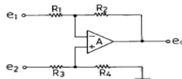
①  $e_0 = e_2 - e_1$                       ②  $e_0 = \frac{R_2}{R_1}(e_2 - e_1)$
